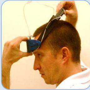
Center the ARES over your nose and slightly above your eyebrows. Remove any hair from under the sensor to ensure that the sensors make complete contact with your skin.
