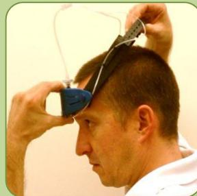
2. If the green light in front of the ARES is illuminated, turn the ARES "OFF". If the light is no longer illuminated, the ARES has automatically stopped recording.
